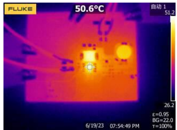
Figure 23. Thermal, 48VIN, 12Vout, 1A
