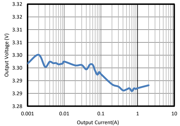
Figure 5. Load Regulation (VIN=12V, VOUT=3.3V)
