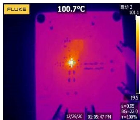
Figure 22. Thermal, 12 VIN, 1 Vout, 8A
