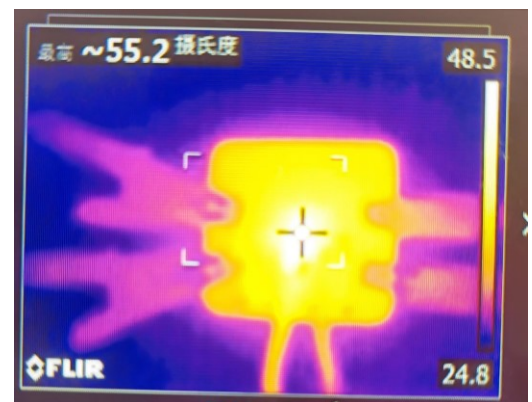
Figure 20. Thermal, 12VIN, 3.3Vout, 3A(SOT563)
