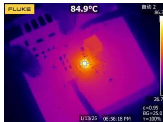
Figure 23. Thermal, 48VIN, 5VOUT, 2A
