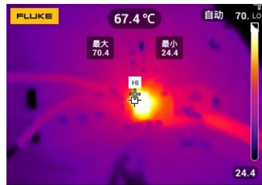
Figure 22. Thermal, Fsw=2.2MHz, Iload=6A
