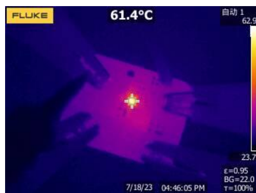
Figure 20. Thermal, V_{IN}=5V , V_{OUT}=1.2V , I_{LOAD}=3A
