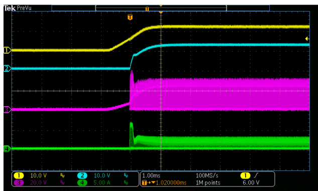
Figure 33. Power up ( I_{LOAD}=1A ) CH1: VIN; CH2: VO; CH3: SW; CH4: IL
