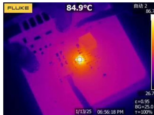
Figure 22. Thermal, 48V IN , 5V OUT , 2A
