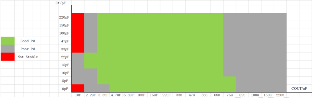
Figure 25. SCT71801A00 Feed Forward Capacitors recommend( R_2=100k\Omega, V_{OUT}=1.8V )
