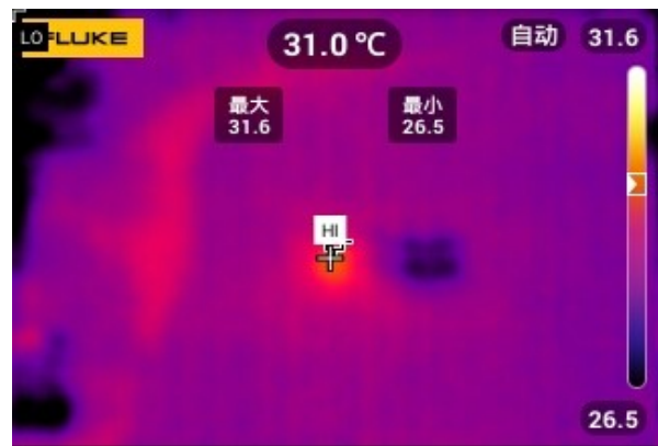
Figure 20. Thermal, V_{IN}=3.3V , V_{OUT}=1.2V , I_{LOAD}=0.6A
