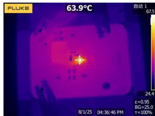
Figure 21. Thermal, 12V IN , 5V OUT , 2A
