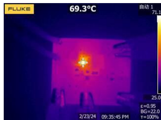
Figure 29. Thermal, 24VIN, 5VOUT, 0.8A
