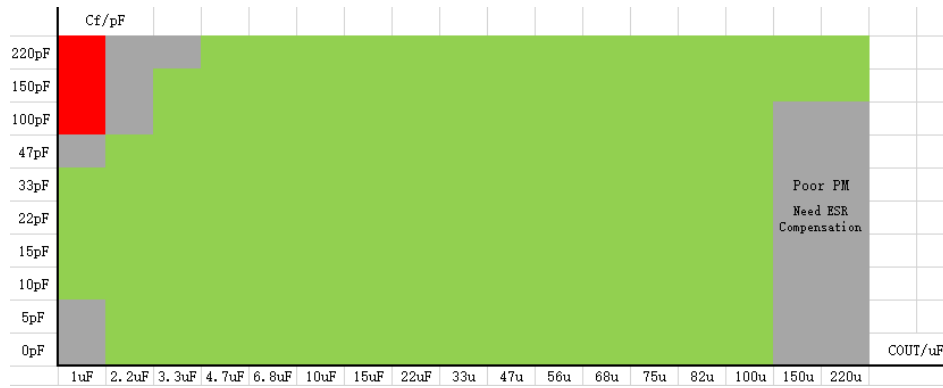
Figure 25. SCT71010A00Q Feed Forward Capacitors recommend(R2=10kΩ,VOUT=1.8V)
