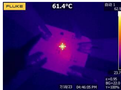
Figure 20. Thermal, V_{IN}=5V , V_{OUT}=1.2V , I_{LOAD}=3A
