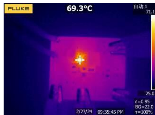
Figure 29. Thermal, 24V IN , 5V OUT , 0.8A
