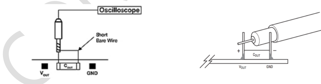
Figure 2. Measuring Voltage Ripple Across Terminals or Directly Across Ceramic Capacitor
