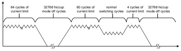
Figure14. Hiccup Mode Protection
