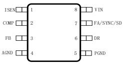
Top View: 8-Lead Plastic MSOP 3mmx3mm
