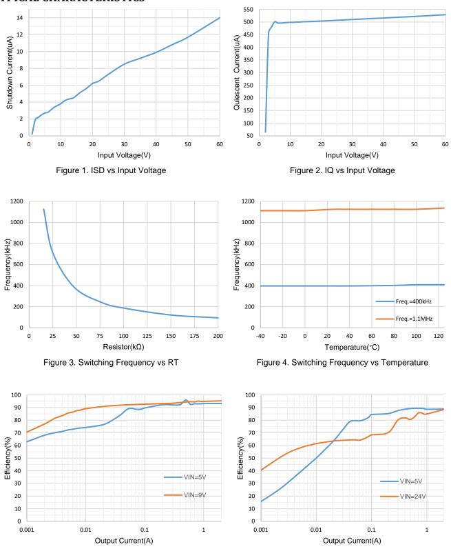
Figure 5. Efficiency vs Load Current, Boost, VOUT=12V
