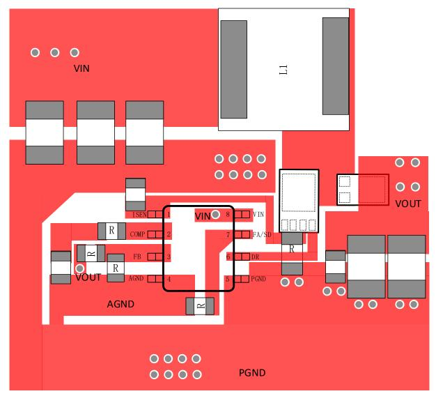
Figure 34. BOOST PCB Layout
