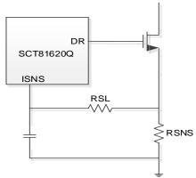
Figure13 .External RSL to increase slope compensation
