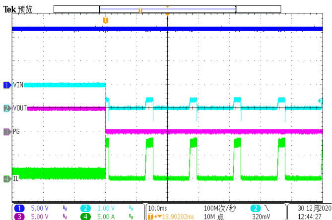
Figure 15. Over Current Protection(1A to hard short)
